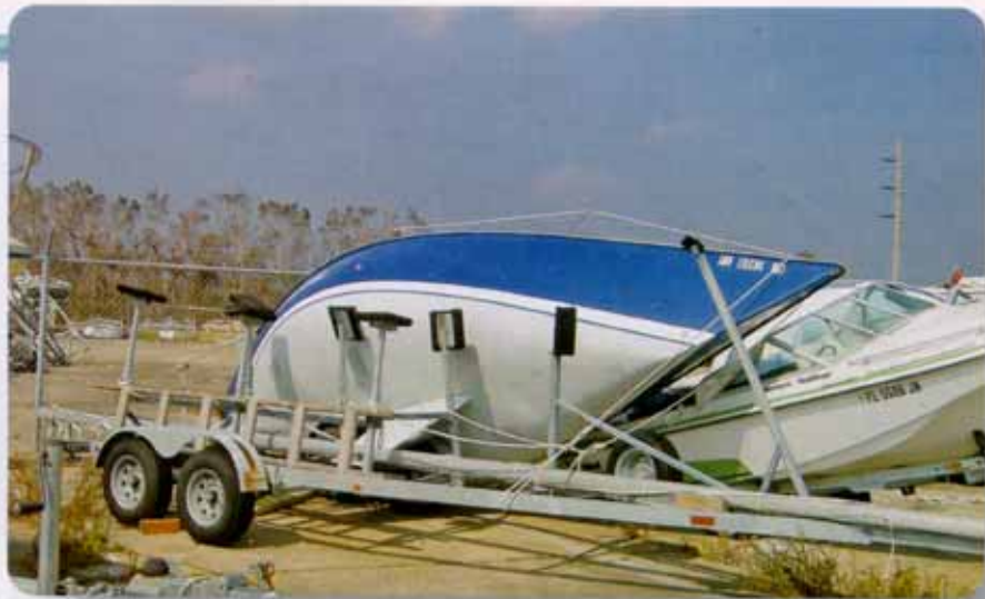
Sailboats with deep keels are vulnerable on trailers, which are too narrow to provide adequate support when the wind is on the beam. Whenever a deep-draft sailboat is stored on a trailer, jack stands should be used to provide additional support.
